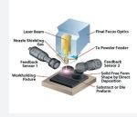
**Direct energy deposition.** A thermal-energy process that fuses material by melting it. Unlike in powder bed fusion, here the powder flows through a nozzle and is melted by the beam as the printer deposits it on the surface of the part being built. This process is also known as laser cladding, laser metal deposition, or electron-beam-directed energy deposition (when an electron beam is used instead of a laser).
