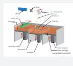
**Powder bed fusion.** A thermal-energy system employing a laser. The laser melts the outline of the part into a thin powder layer. Another powder layer is then spread onto the first layer and the laser melts the part's outline again. This process is repeated layer by layer until the part is complete and can be lifted out of the (now filled) powder bed.
